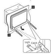
2 When the lower level is removed, remove from the upper two catches of the trim plate (6).
