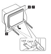
2 When the lower level is removed, remove from the upper two catches of the trim plate (6/7).
