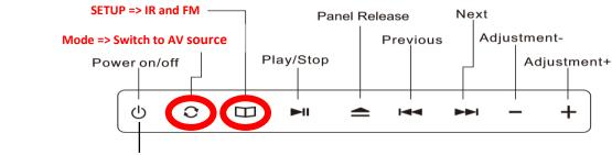
Hold the power icon for "2 seconds" to switch off power
